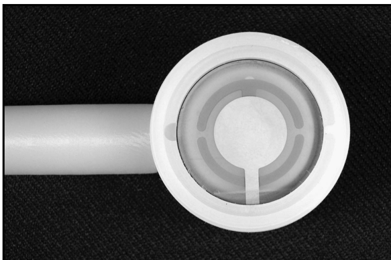
Figure 9. Crystal in place with correct electrode orientation.
