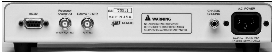
Figure 2. Back Panel of QCM200 Digital Controller.
